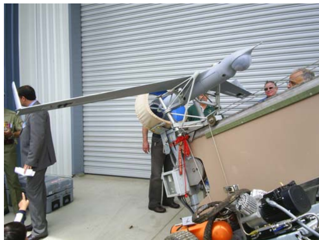
“Scaneagle” on its launching ramp
