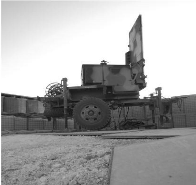
AN/TPQ-36 Antenna in position – Iraq 2005
